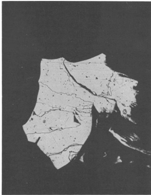
Figure 1 Cleavage facet, \times 44 .
